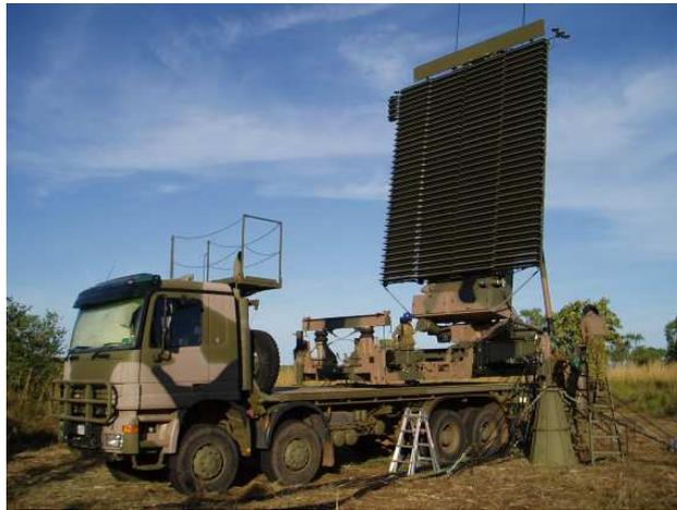
TPS-77 Air Surveillance Radar operated by 114MCRU at Darwin
